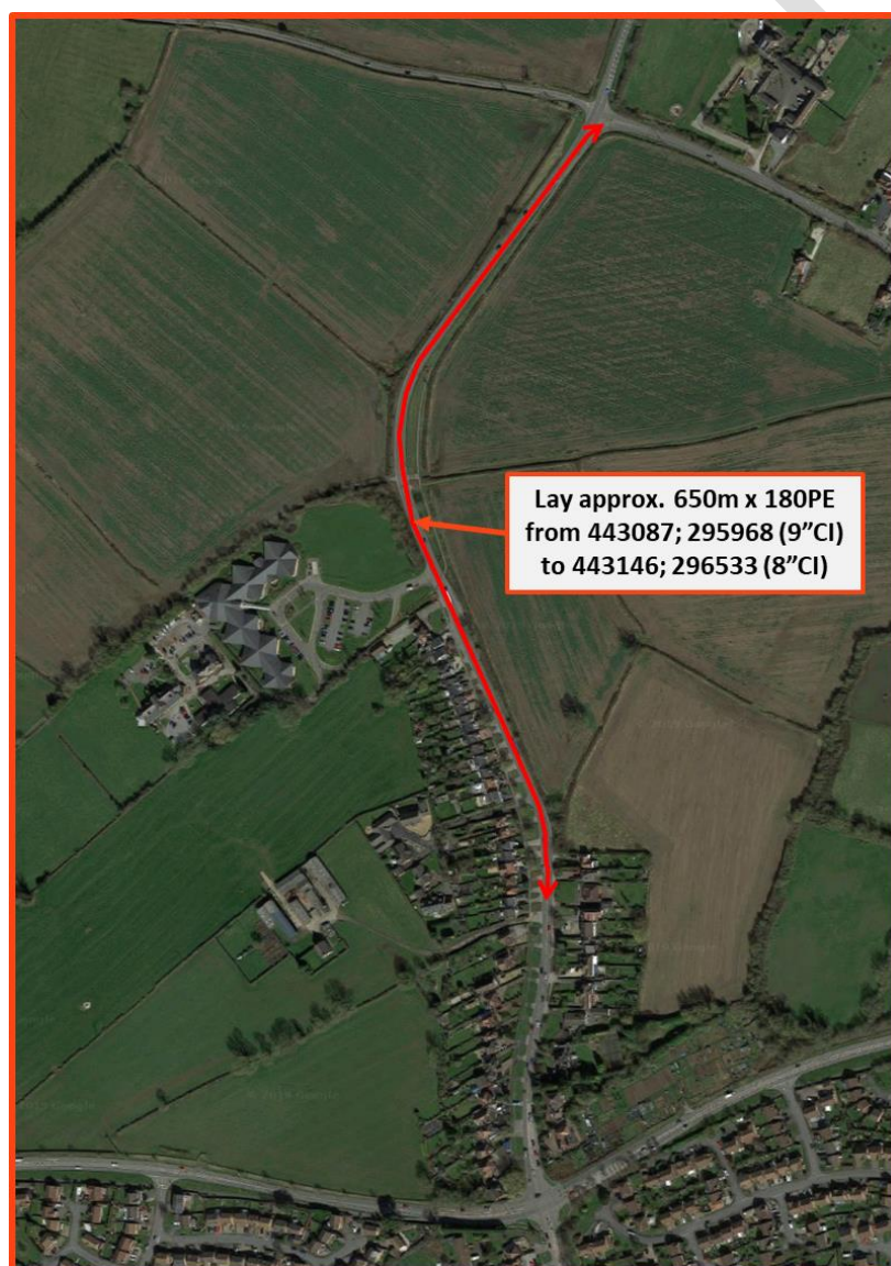
Figure 11 – Contiguous reinforcement to maintain 23mbar
