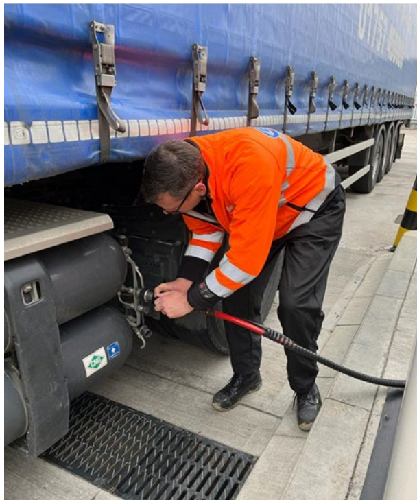
Figure 9: Vehicle fueling with CNG
