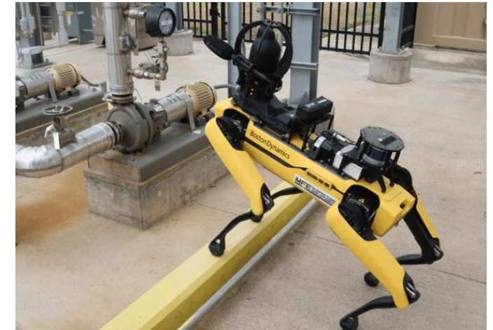
Boston Dynamics' Spot robot dog equipped with various sensors to autonomously detect leaks.
