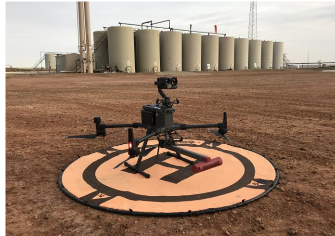
A SeekOps sensor attached to a drone to survey a site following a preplanned flight path.
