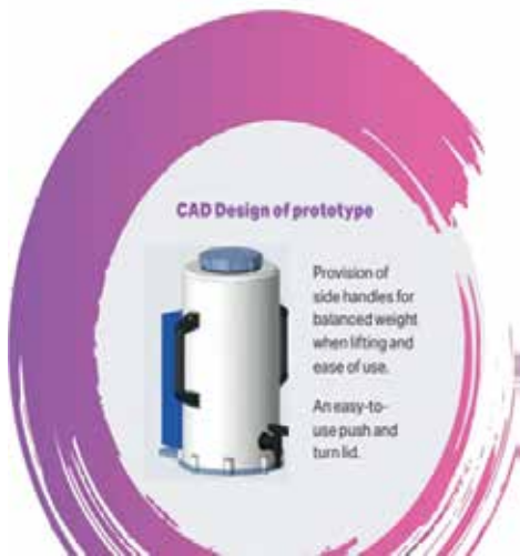
Figure 16: Low Power Hot Water prototype
