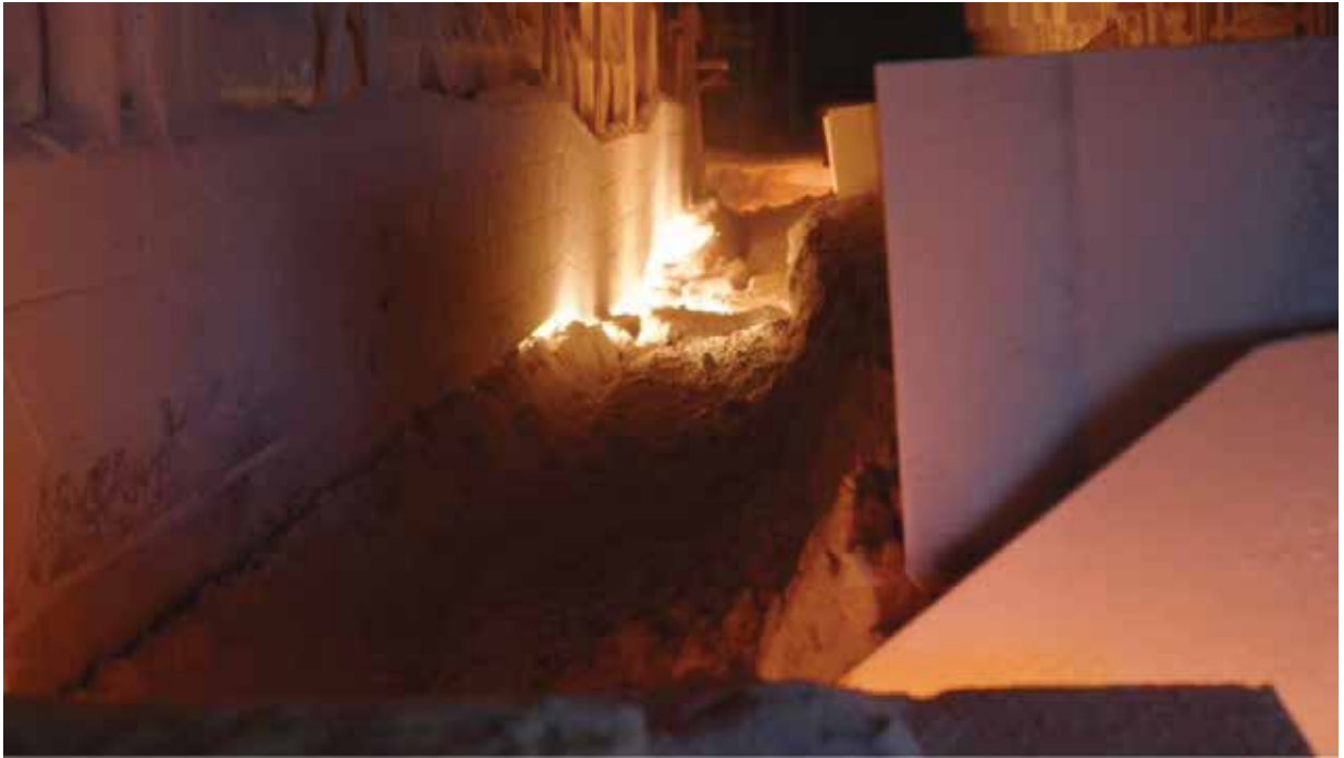
Figure 11: Example of high energy consumer seeking to use Hydrogen in the future: Pilkington's glass - the raw materials entering the furnace
