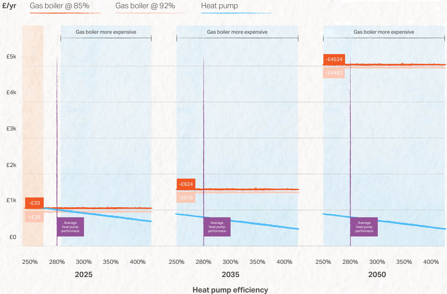
Figure 9: Heat pump vs gas boiler running costs at various performance levels over time under 'shift to gas' approach
